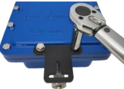
5. Tighten the bolts to 11 ft-lbs. Do not overtighten.
