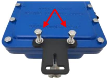
4. Add the (2) 5/16 bolt flat washers (supplied) as shown below and replace the bolts.
