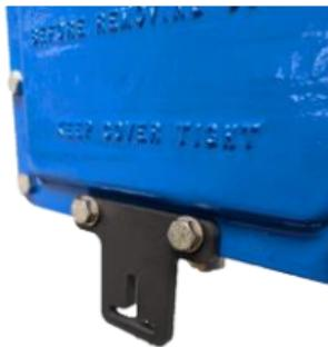
6. The Stowage Plate can now be used to properly stow the ground clamp
