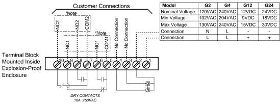
\*NOTE: NO: NORMALLY OPEN CONTACT THAT <u>CLOSES</u> WHEN GROUND IS ESTABLISHED NC: NORMALLY CLOSED CONTACT THAT <u>OPENS</u> WHEN GROUND IS ESTABLISHED
